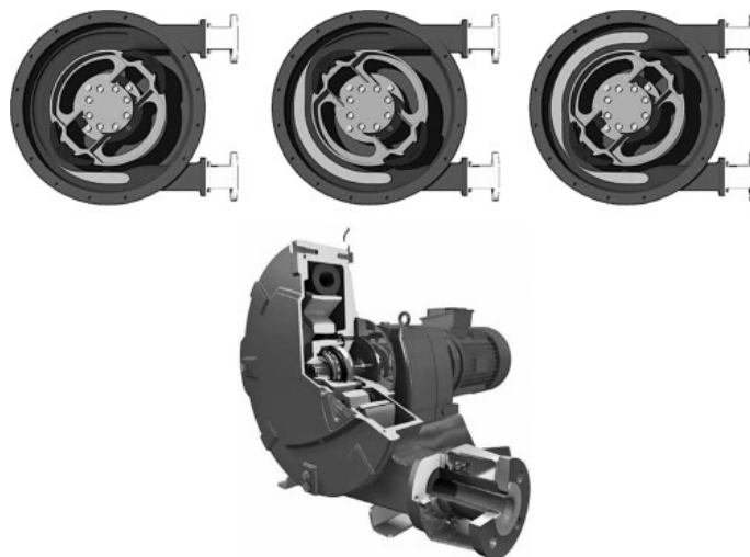
Fig. 6 Schematic diagram for a peristaltic pump. [3]
