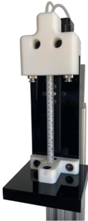
Fig. 11 A view of the actual machine that shows the resin mixing assembly.
